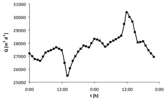
Fig. 2. Variation of the influent wastewater flow rate at the WWTP.
