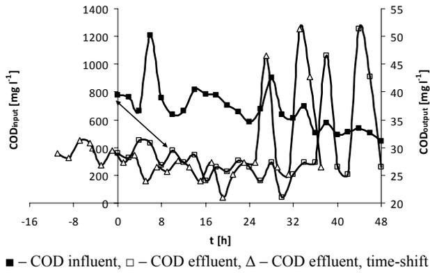
Fig. 4. Visualization of time-shift between the WWTP input and output.
