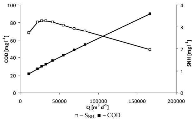
Fig. 10. Influence of wastewater flow rate on effluent COD and SNH concentrations.
