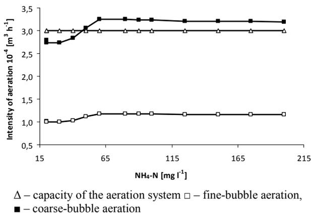
Fig. 7. Influence of influent ammonium nitrogen content on the intensity of aeration for coarse-bubble aeration and fine-bubble aeration systems.
