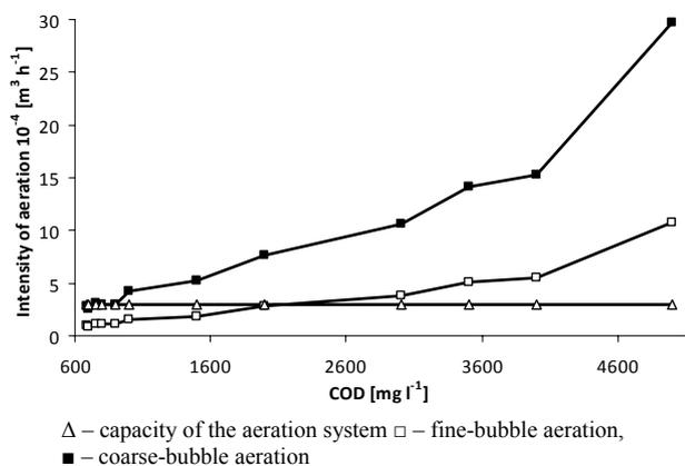
Fig. 5. Influence of influent COD value on the intensity of aeration for coarse-bubble aeration and fine-bubble aeration systems.
