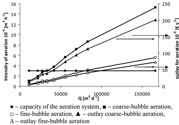
Fig. 9. The intensity of aeration and costs for oxygen supply for coarse- and fine-bubble aeration on different wastewater flow.
