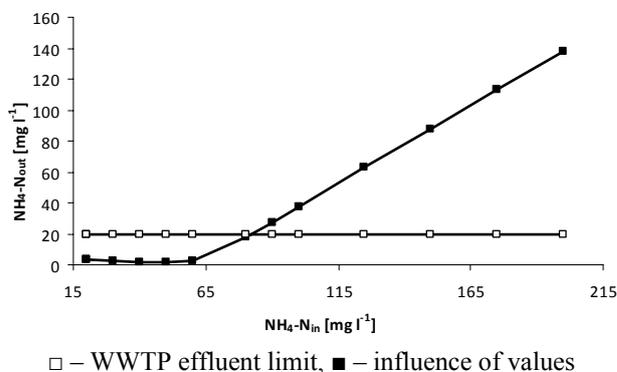
Fig. 8. Influence of influent ammonium nitrogen concentration on effluent ammonium nitrogen concentration.
