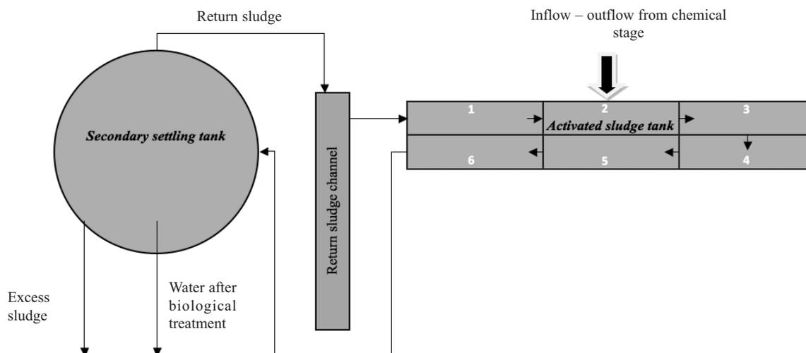
Fig. 1. Layout of the biological stage of the WWTP.
