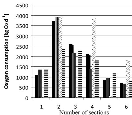
Fig. 13. Oxygen profiles and corresponding oxygen consumption for three aeration scenarios.
